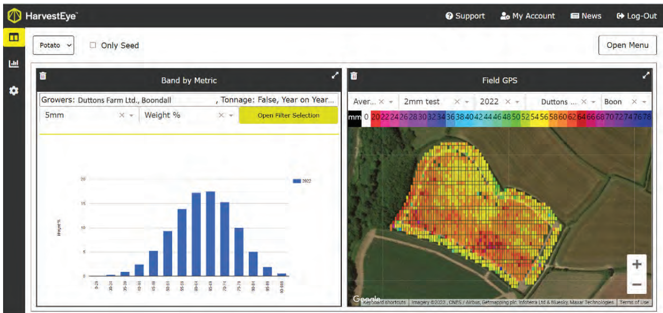
The HarvestEye system can provide detailed information on tonnage by size band, as well as distribution of different sizes within the paddock.
