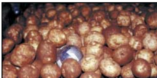
The instrumented sphere at work
