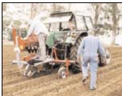
Planting at Warragul, Victoria with a fully automatic transplanter
