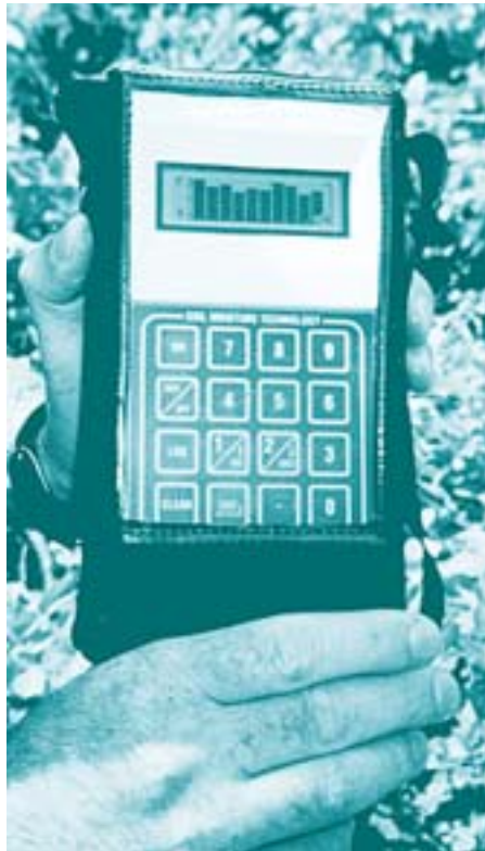
The Gopher can graph water use patterns in the field.
