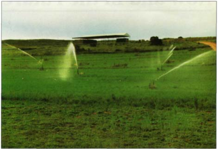
Cans were placed under the irrigation system to calculate the distribution uniformity
