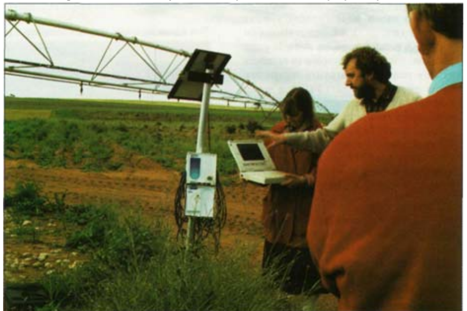
Downloading the EnviroSCAN system in the paddock with a laptop computer
