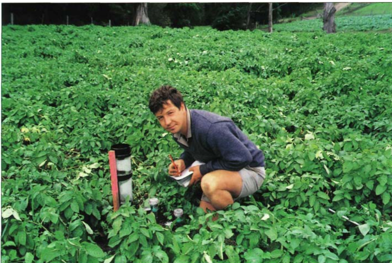
Robertson potato grower Rodney Mauger recording rainfall and tensiometer readings.
