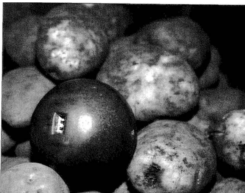
FIGURE 1: Instrumented sphere, often called a pseudo-fruit/vegetable, is proving to be a useful tool in identifying handling problems.
