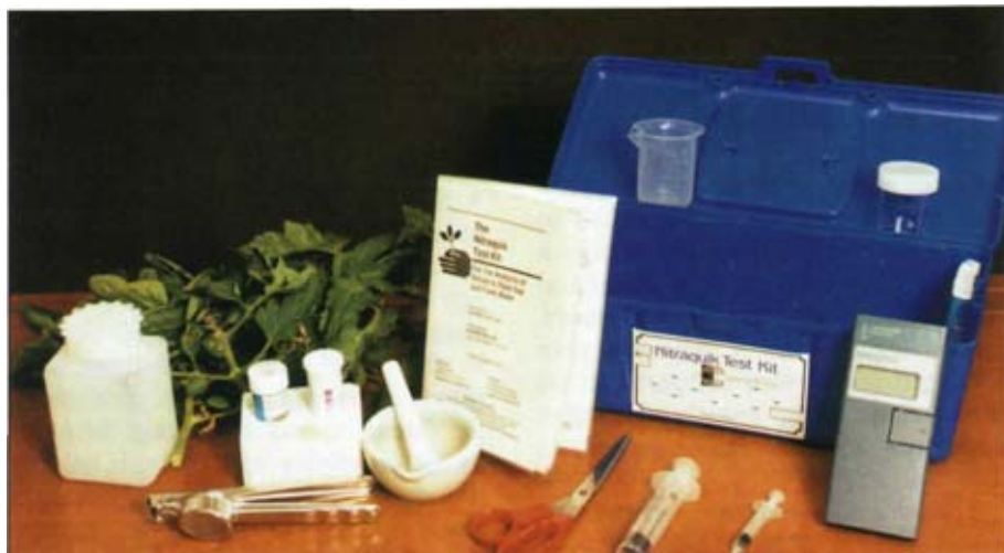
Components of the Nitraquik Sap Test Kit (garlic crusher, syringes, beaker, Nitrachek meter, Merck ® test strips and standard nitrate solution).
