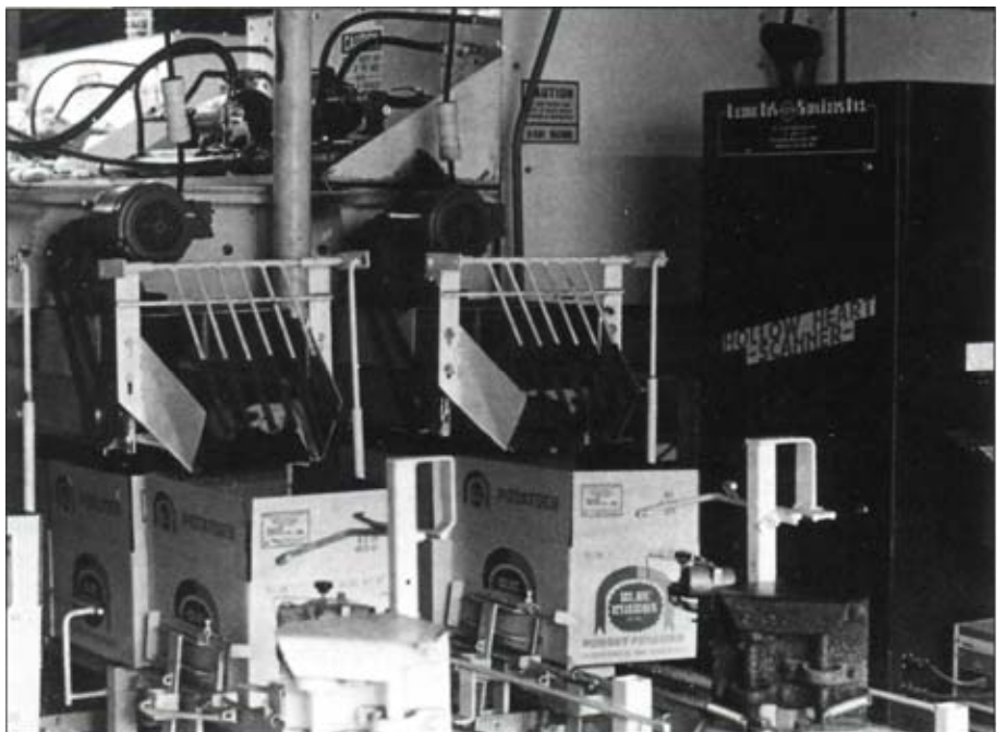
A hollow-heart scanner in use in a fresh market packhouse in the USA.
