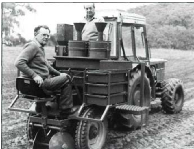
The new SA Department of Agriculture trial potato planter is 3 point linkage mounted. Ross Allen (standing) and Merv Schubert (seated) designed and built the machine.
