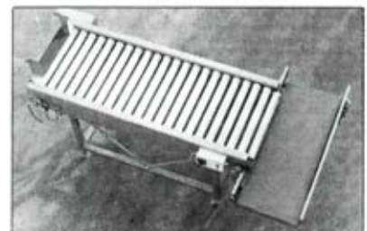
FINAL GRADE INSPECTION TABLE WITH REVERSIBLE CROSS CONVEYOR.
