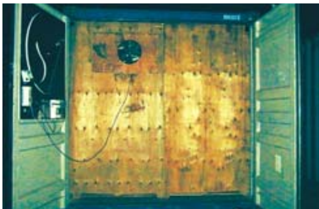
Door end of a 'one-trip' Pot-Tainer conversion of a P&O-type onion Fantainer showing how the fan has been relocated from the door. The fan is now mounted in a temporary plywood bulkhead inserted after the container has been loaded with potatoes packed in jute bags on a layer of pallets. Note that the bottom of the bulkhead is cut away to allow air to return to the loadspace. A panel holding the control equipment and rotary damper (to regulate the rate of air freshening) has been fitted over the original fan opening in the left-hand door.
