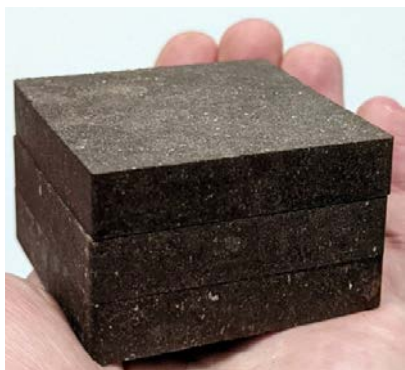
Block of 'StarCrete', made from potato waste, salt and dust. (Image: designboom)
