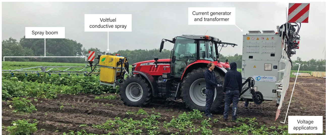
Figure 1. The CROP.ZONE system combines a conductive spray with electrical applicators
