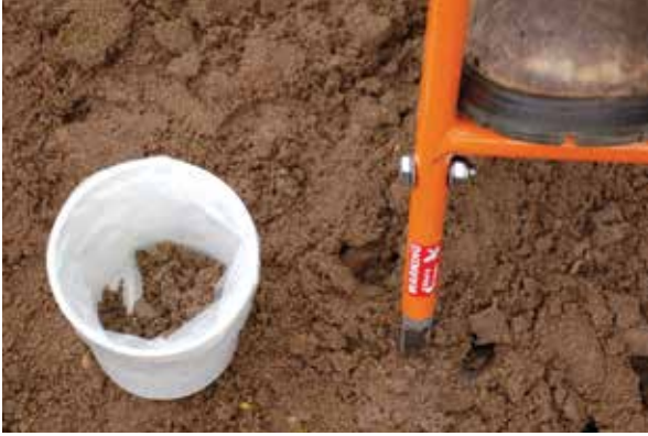
Corer used to extract soil samples for testing. Image from SARDI
