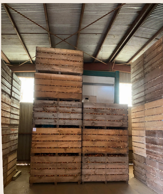
Figure 20. The Tolsma drying wall for curing freshly harvested/cut seed potatoes (left) and the Tolsma open space ventilation and cooling system (right). Images supplied by Tolsma.
