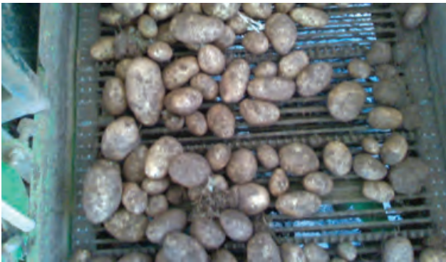
The HarvestEye system uses AI to separate potatoes within an image, then applies an algorithm to estimate size and weight.
