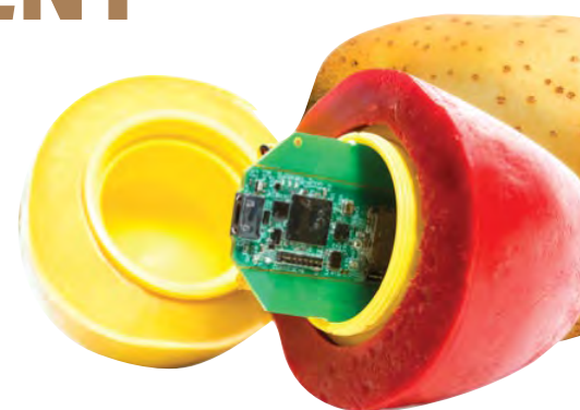
Figure 6. The SmartSpud consists of an accelerometer mounted inside a potato-shaped urethane capsule.
