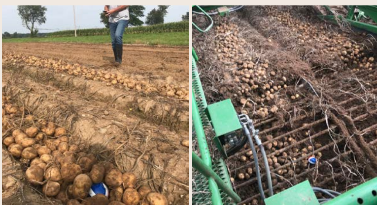
Figure 10. Impact recorders can be used to identify points on the harvester where consistently high impacts occur, then test ways to reduce these impacts. Image: P. Morris, Techmark
