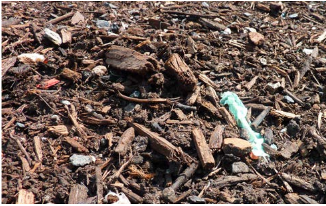
Figure 2. Any delivery of RO or compost must be checked to ensure it is free of contaminants such as plastic and glass.
