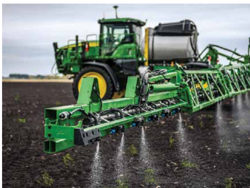
See and Spray unit from John Deere
