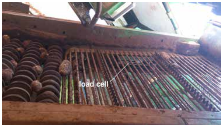
The yield monitoring system has a cabin-mounted operational recording terminal that connects to the yield sensor (load cell mounted under the final delivery belt) and a GPS.
