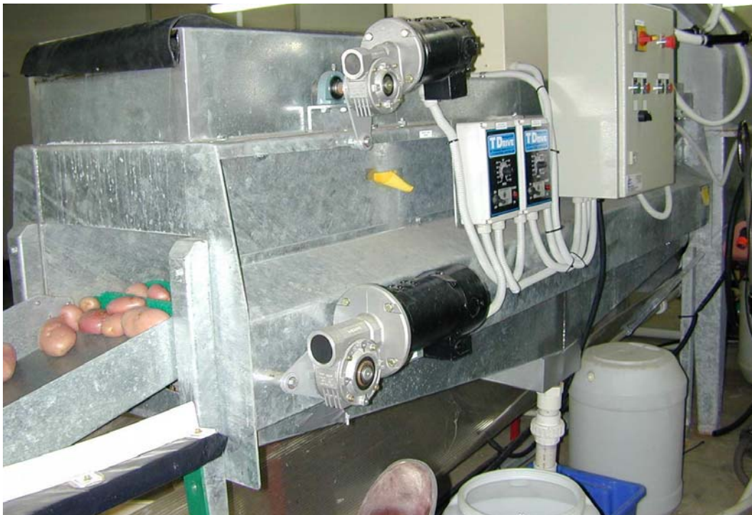
Figure 2 Mini Potato Washing Plant – control panel.
